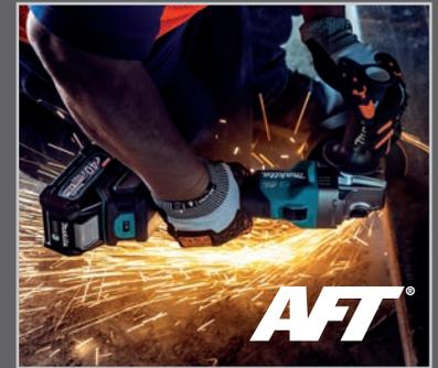
Active Feedback-sensing Technology (AFT®) turns the motor off if rotation of the wheel is suddenly forced to stop.
