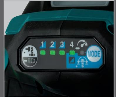
4-speed power selection switch for a wide range of applications.
